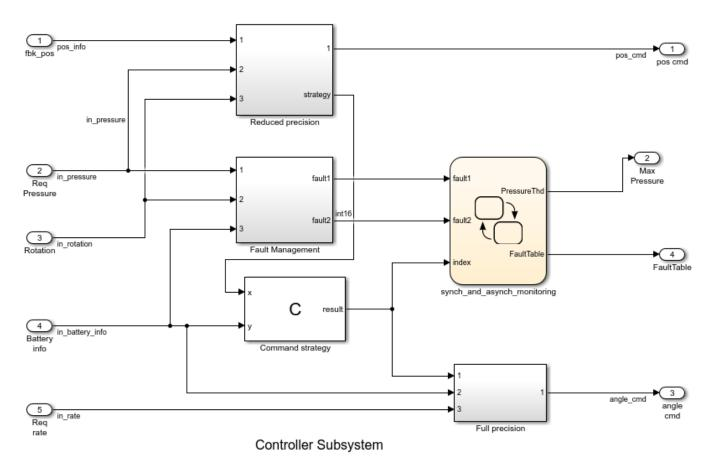
The Command Strategy block implements a look-up table using custom C code and outputs a value result based on two inputs x and y.
