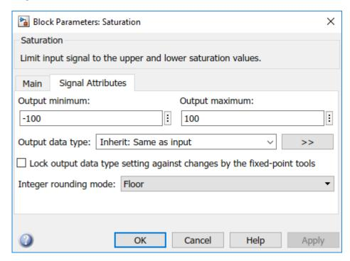
Note that specifying a lower and upper limit on the **Main** tab of the Saturation block is not sufficient to constrain the signal for the Polyspace analysis. The analysis uses the design ranges specified on the **Signal Attributes** tab.
