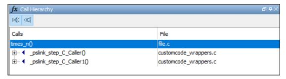
Select one of the wrapper functions to open the source code for customcode\_wrappers.c.
