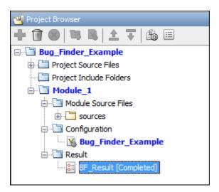
The Bug Finder (Code Prover) results are stored in a .psbf (.pscp) file in the results folder. For instance, if you save your project in C:\Projects\, a .psbf file for the Bug Finder analysis results on the first module Module\_1 is stored in C:\Projects\Module\_1\BF\_Result. See also "Contents of Polyspace Project and Results Folders" on page 2-10.
