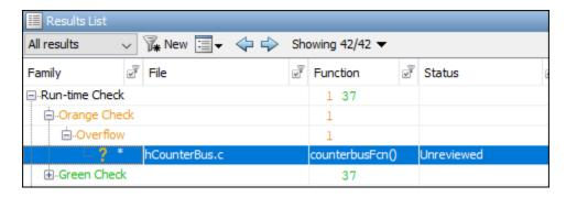
The check highlights an addition operation in the counterbusFcn function that can overflow:
